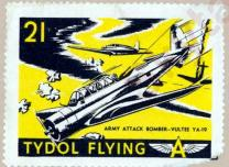
This all-metal high-speed attack plane is used by the Army for low-altitude ground straffing and bombing. The pilot and gunner are seated in tandem. The third member of the crew, the bombardier, rides in a rear compartment provided with a retractable gun platform in the bottom of the fuselage. Here he can protect the ship from rear attack while his shipmates operate four heavy-caliber machine guns forward.
