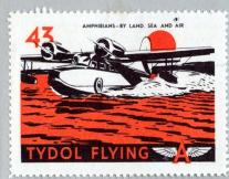
An aircraft able to land on either water or land, has a distinct advantage. Modern high performance amphibians such as the "Grumman-21," used by the Coast Guard and private owners, are a combination of the fuselage of an airplane and the seagoing hull of a flying boat equipped with retractable landing wheels. The engines are placed high on the wing to keep the propellers clear of spray when maneuvering on water. Amphibians perform well as either land or seaplanes.
