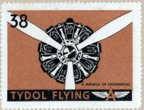
When you drive a car 45 m.p.h., the engine turns at about 3,000 revolutions per minute. A Flagship's engines at cruising speed, however, turn only 1,800 rpms, or nearly half as fast. Great power at low crankshaft speed is one reason why modern aircraft engines rarely fail in spite of light construction. Compare the Wright Brothers' 16 pounds per horsepower engine, to the one pound per horsepower Curtiss-Wright "Cyclone" engines which drive the Flagships.
