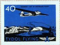
Soaring aircraft are launched from hilltops or level ground by man power, or by a "winch" which reels in a long tow cable attached to the sailplane. As the craft gains air-speed, it rises at the end of its tow cable like a giant kite. The pilot then "cuts loose" and sails away, gaining additional altitude by maneuvering in currents of rising air found beneath cumulous clouds, along ridges, hills or sand dunes. Soaring in the U. S. is conducted by the American Soaring Society.
