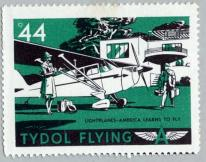
The "lightplanes"—small, 2-place cabin monoplanes powered by 50-h.p. engines, are America's most popular aircraft. Several airplanes of this type are priced between \$1,000 and \$2,000 new. Such little ships are extremely stable; cruise around 80 m.p.h.; and cost less to operate than the average car—from 1½ to 2c per mile. Any good automobile driver with normal vision should be able to fly a lightplane solo after eight hours of instruction. Lessons cost about \$10 an hour.
