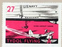
Before America's airship program was curtailed, the Navy developed the airplane hook-on technique to a high degree of efficiency. In 1935, the Airship Macon carried five speedy airplanes within her huge hull. Such an airship, helium-filled and fireproof, equipped with scouting airplanes, operates as a high-speed aircraft carrier, with the added advantage of being invulnerable to mines, torpedoes, attacks from submarines, battleships and other hazards.
