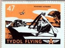
Three years ago the government sponsored the development of an experimental "Roadable Autogiro," a unique aircraft designed to meet the flying limitations of the average man. The engine is connected to the landing gear by a transmission, so that when the autogiro rotor is folded back the little machine can travel on the highway with automobile traffic. The experimental machine flies at 90 m.p.h. takes off in 40 feet, and can land vertically in confined spaces.
