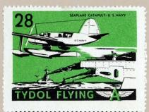
U. S. cruisers and capital ships carry seaplanes to scout the enemy and direct the fire of the big guns. As seaplanes cannot safely take off from the rough water of the open ocean, our Navy developed the launching catapult. The seaplane's float rests in a cradle on wheels. The pilot opens the throttle, gives a signal and the airplane is shot along the track reaching full flying speed in only 60 feet. The seaplanes sometimes drop alarmingly, but seldom touch the water.
