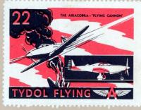
The most deadly warplane today is believed to be the Army's newest pursuit ship with the tricycle landing gear, the Airacobra. Its sleek nose houses a 37 mm. cannon which fires high explosive shells. The muzzles of 4 machine guns sprout from its stubby wings. The 1000 h.p. liquid-cooled engine behind the pilot's seat will drive the ship over 400 m.p.h. to a height of 7 miles above the earth. Such a ship has no foreign equal.
