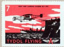
Eugene Ely first demonstrated the practicability of naval aircraft by flying his Curtiss biplane from shore to a small platform on the deck of the cruiser "Pennsylvania." The arresting gear improvised to stop the plane, once it landed on the platform, consisted of a row of sandbags connected by ropes athwartship which were picked up by a drag hook attached to the airplane. After his successful landing before high-ranking Naval obervers, Ely took off and flew back to shore.
