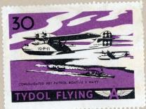
During recent Caribbean Fleet maneuvers, one of our Navy's consolidated flying boats is said to have remained in the air for three days continuously—a feat which might enable the same ship to fly across the Atlantic four times without refueling! The speed of the PBY is largely due to the elimination of wind resistance by retracting the wing-tip floats into the wing, once the ship has left the water. Such flying boats are seaworthy and take amazing poundings without damage.
